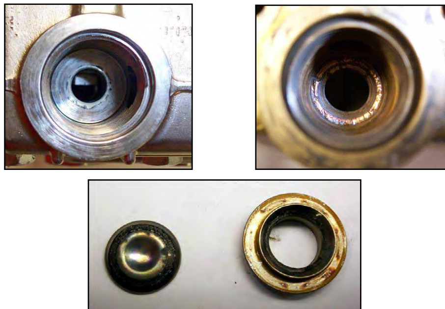
Figure 5-2. Inspect Manifold and Old Valves
