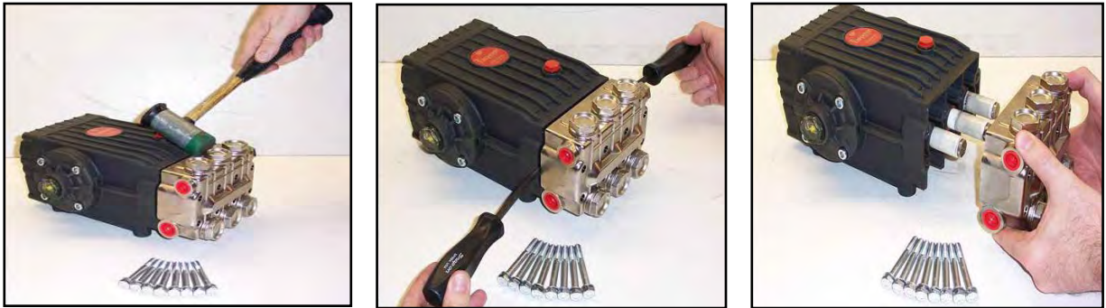
Figure 5-6. Separate Manifold from Crankcase
