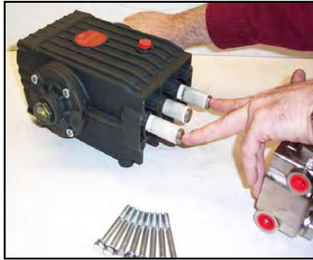
Figure 5-16. Re-install Manifold and Torque Fasteners
